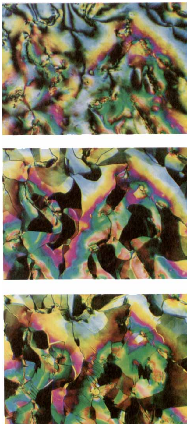
Figure 3. Textures of HEX6. From the upper texture: S_F phase (150°C), crystal G phase (140°C) and crystal H phase (130°C).
